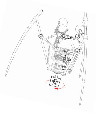
Wind clockwise (from the top view) until you feel that the necessary force increases significantly; do not wind further as this is the sign that the movement is fully wound. You need to wind your TriPod every 8 days.
