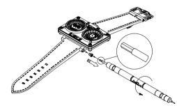
2. Remove the screw on the left-hand lug by turning anticlockwise with the supplied screwdriver.
