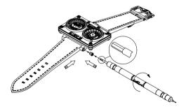
3. Screw-in the left-hand screw in the lug by turning the screwdriver in a clockwise direction. Repeat steps 1-3 on the other side of the case.
